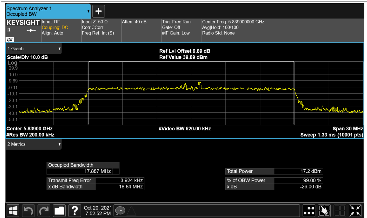
OBW HVHT 5.8G-20M-16QAM 5839MHz Ant2
