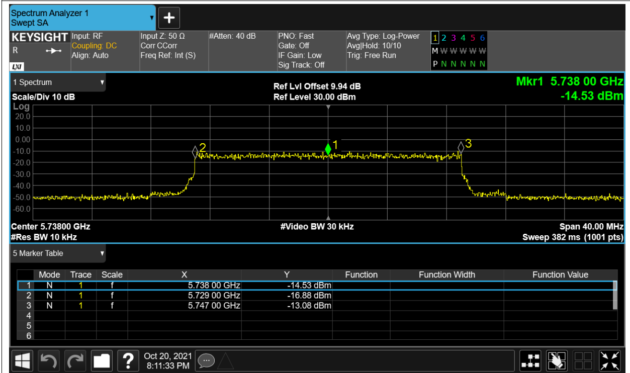
Freq. Stability LVLT 5.8G-20M-16QAM 5738MHz Sum
