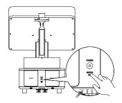
Short press the linking button in the battery compartment of the aircraft, and the linking indicator will flash green quickly.
