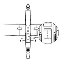
Once linking is successful, the linking indicators both on the base station and the aircraft will flash green slowly.
