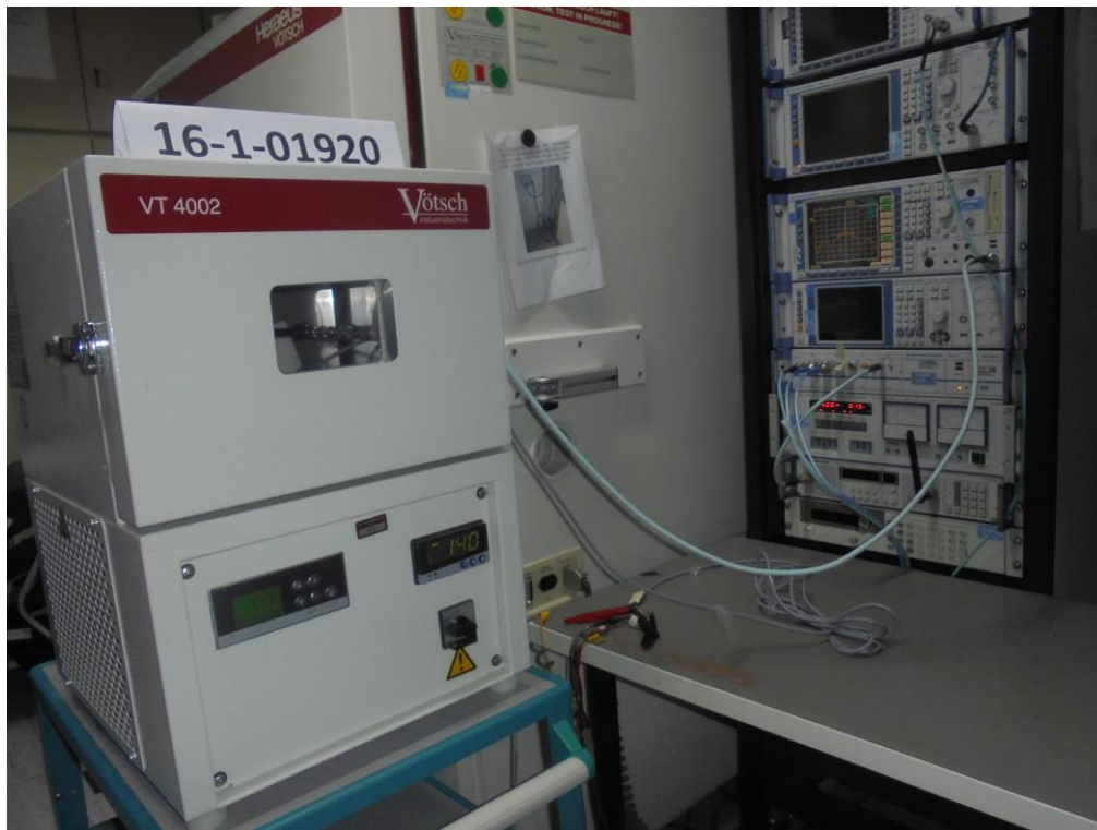
Test setup 3 EUTA+AE1 Complete setup with Temperature Chamber
