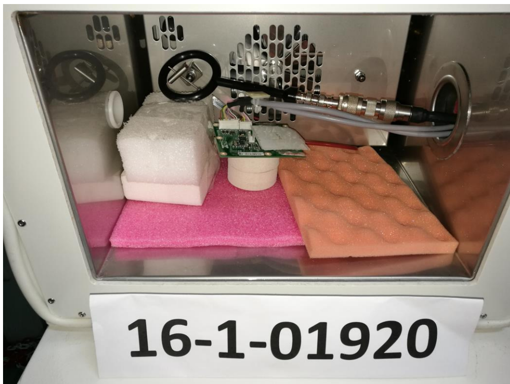
Test setup 3 EUTA+AE1 inside view Temperature Chamber
