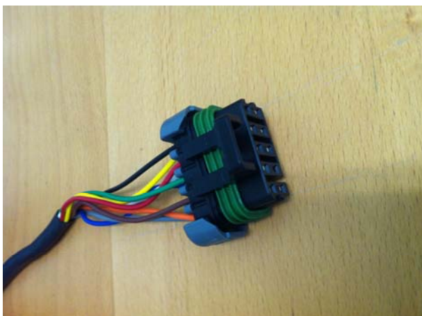
ADIO connector on iBright standard harness
