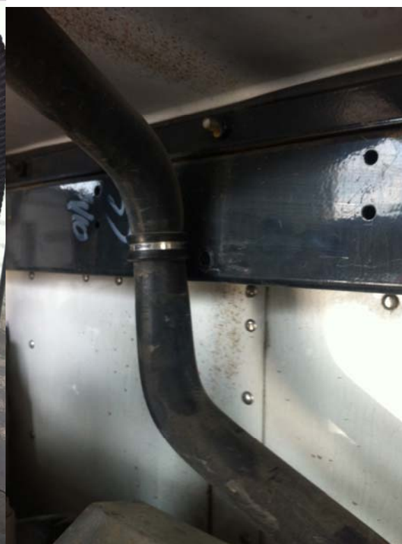
Existing radiator hose clamp needs to be moved one hole to the left
