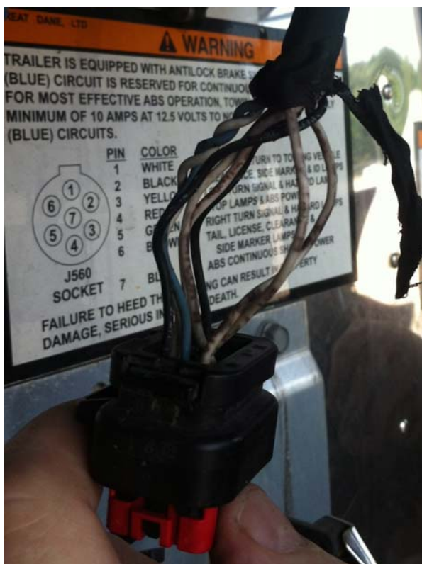
Display connector – unwrap some of the protective tape to get at the wiring.
