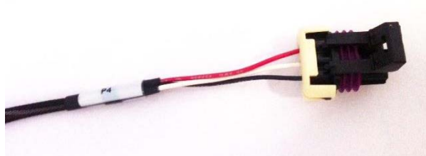
Momentary switch connector on the iBright harness
