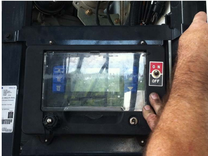
iBright switch and switch plate are to the right of the display.
