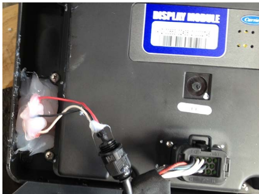
Ibriht switch is completely sealed at the back of the display.
