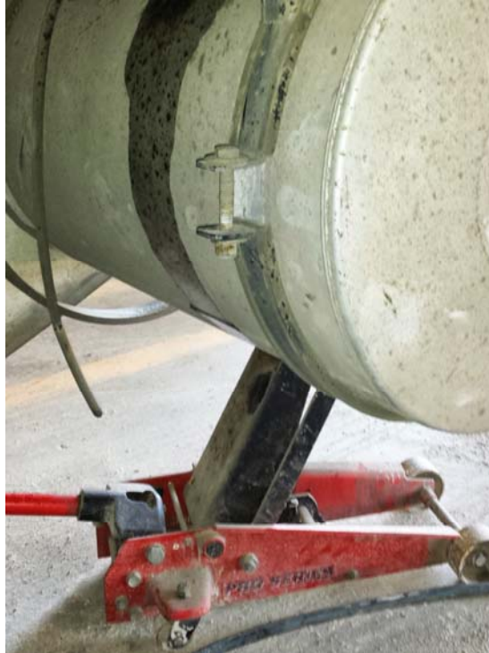
The best way to lift the tank of the mounting brackets is using a jack
