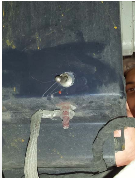
Reefer start/run switch (master switch) on Advance micro relocated to the back of the controller.
