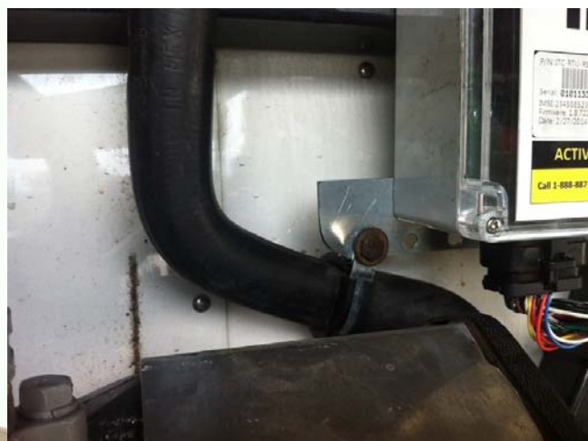
To prevent abrasion use 1 3/8" hose clamp bolted to the iBright bracket
