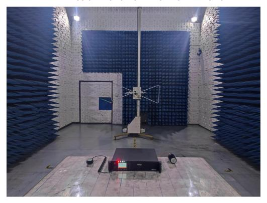
RADIATED EMISSION TEST SETUP ABOVE 1GHz BY AC POWER
