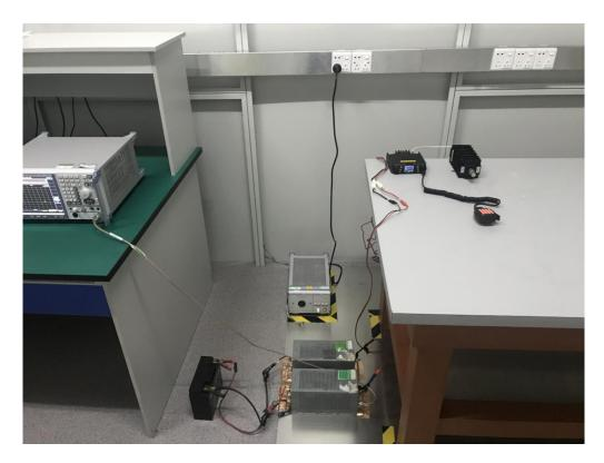
**RADIATED EMISSION TEST SETUP**
