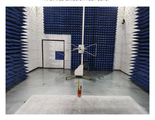
RADIATED EMISSION ABOVE 1G TEST SETUP
