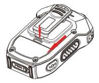
Lift on clip as shown and slide clip down in direction shown to remove
