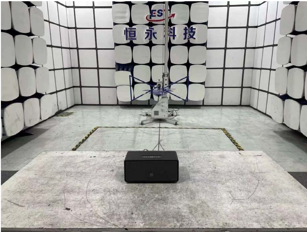
Radiated emission test: Below 1GHz
