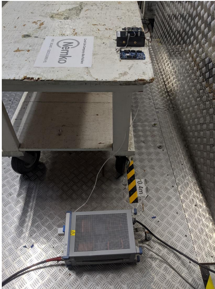
Figure 6 - Conducted AC emissions, side view
