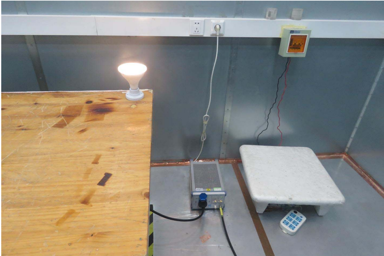
Picture 2: Conducted Emissions Test Setup
