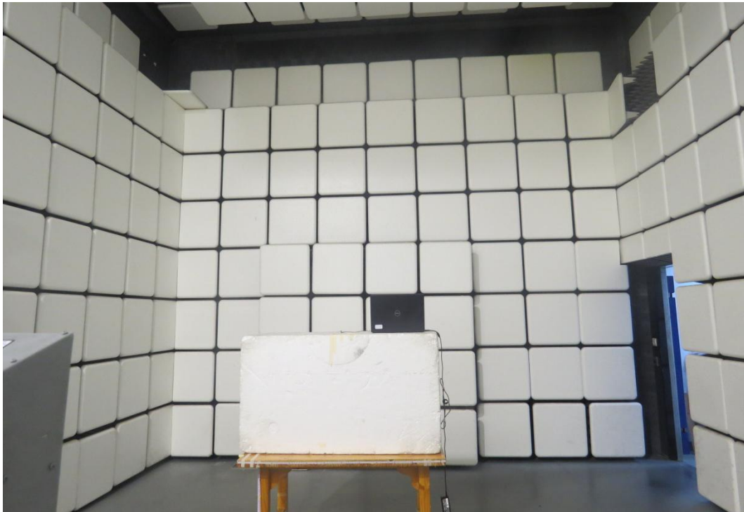
Picture 1 Radiated Emission Test Setup
