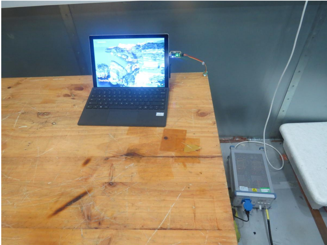
Picture 2 Conducted Emission Test Setup
