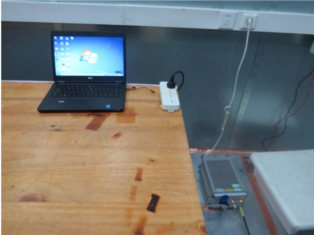
Picture 2 Conducted Emission Test Setup
