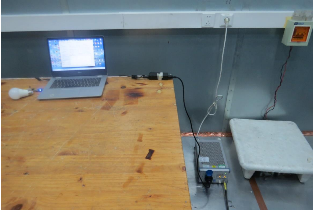
Picture 2 Conducted Emission Test Setup
