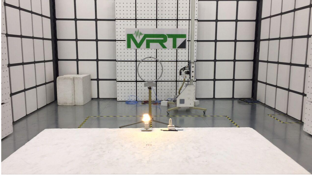
Description: Radiated Emission Test Setup for 9kHz ~ 30MHz
