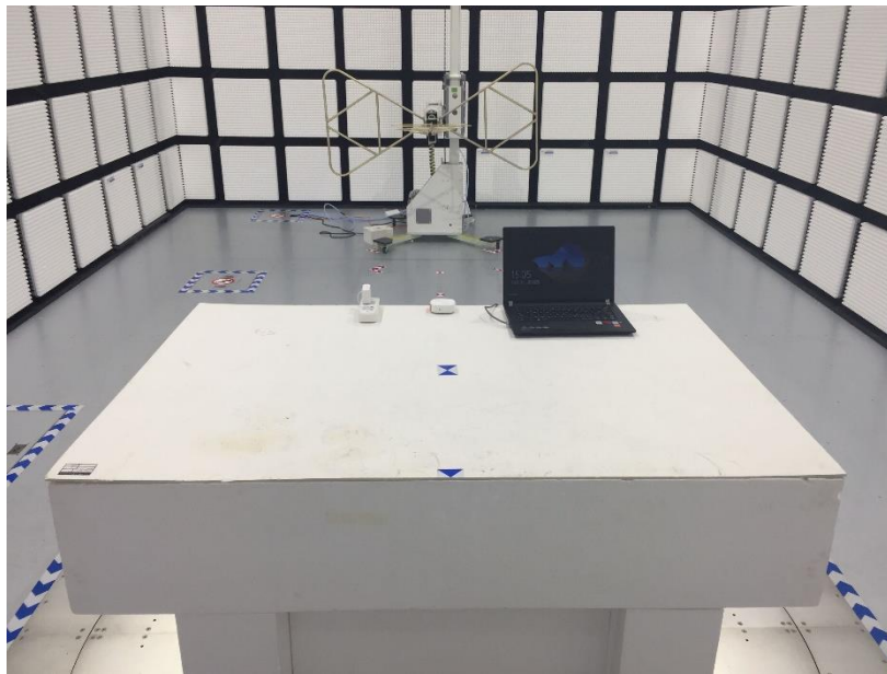
RADIATED RF MEASUREMENT SETUP (ABOVE 1 GHz)
