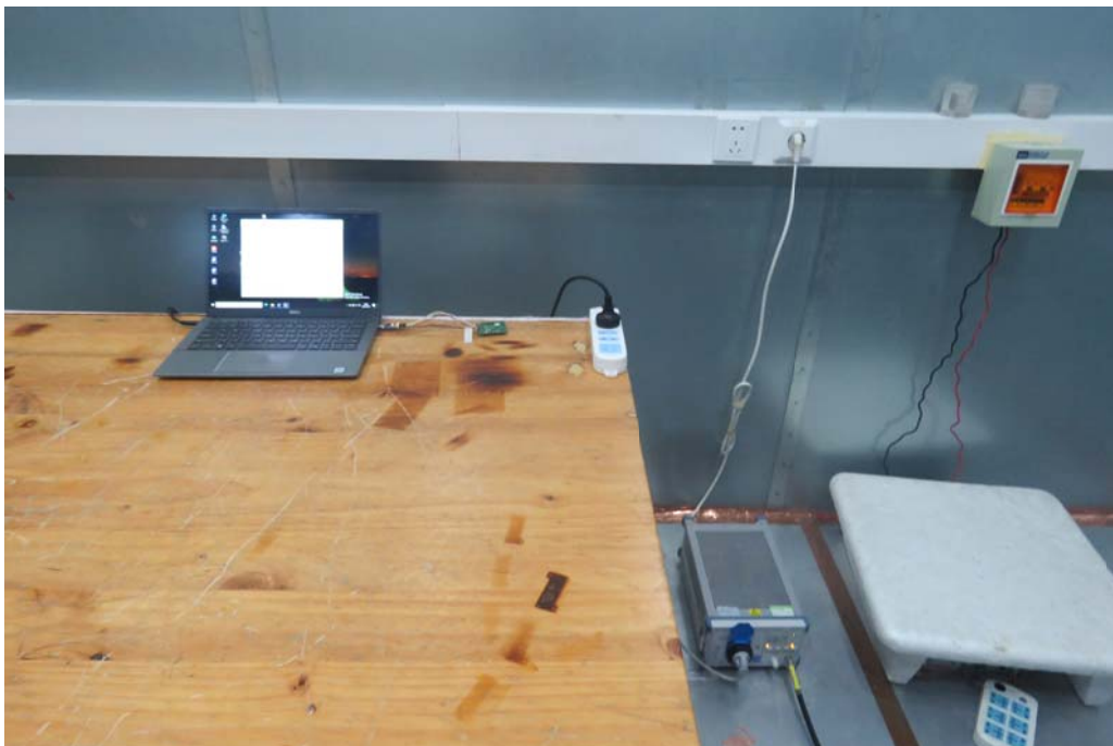
Picture 2 Conducted Emission Test Setup
