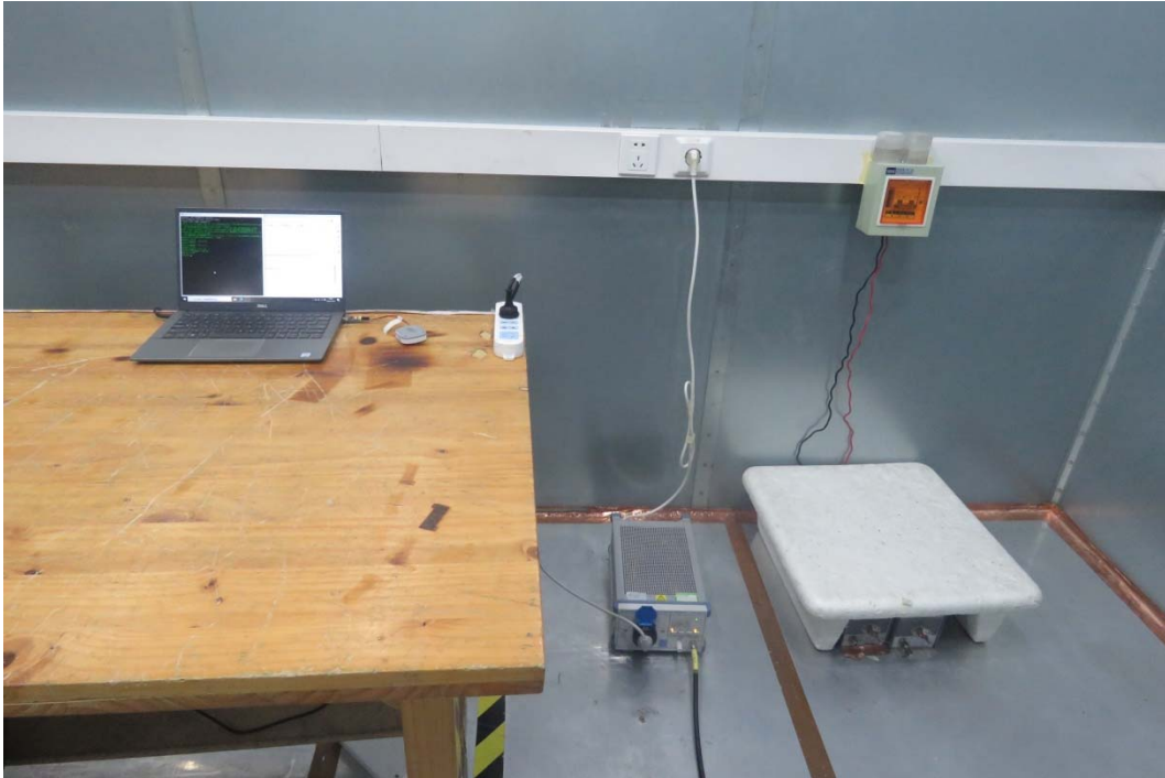
Picture 2 Conducted Emission Test Setup
