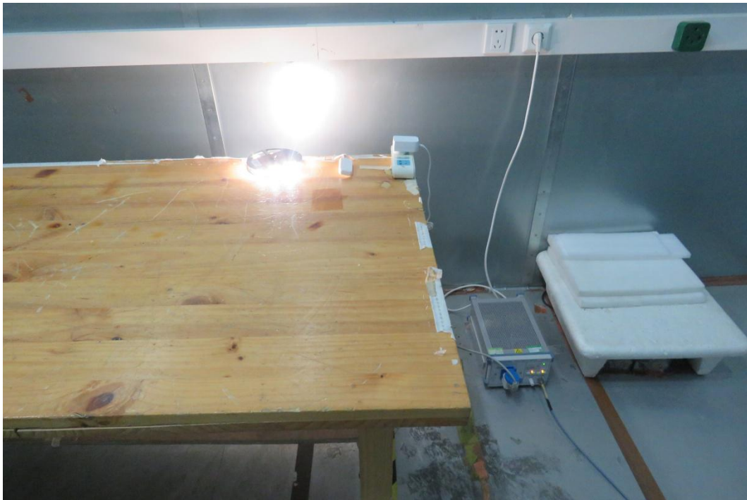
Picture 3 Conducted Emission Test Setup
