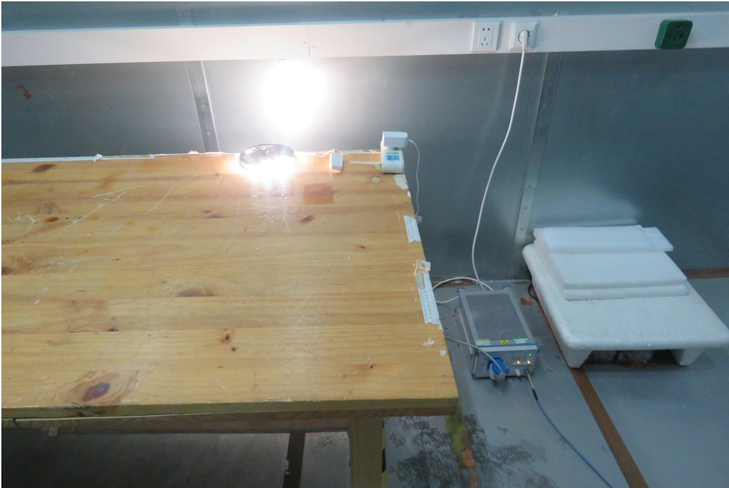
Picture 3 Conducted Emission Test Setup
