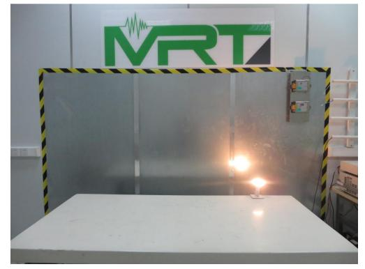
Description: Front View of the Conducted Emission Test Setup for 0.15kHz ~ 30MHz
