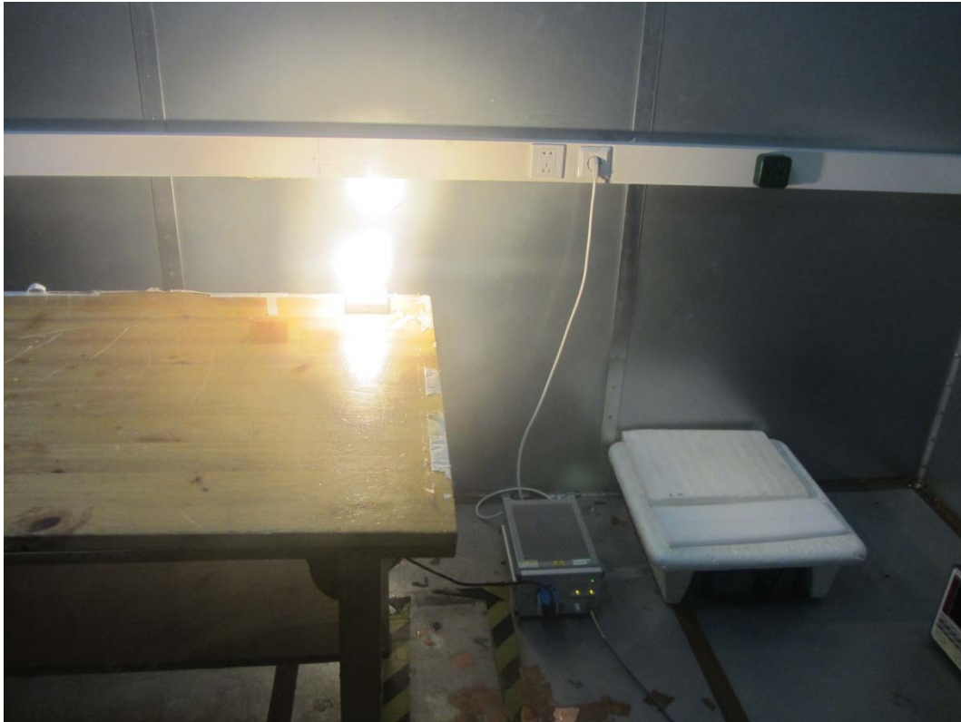
Picture 3 Conducted Emission Test Setup
