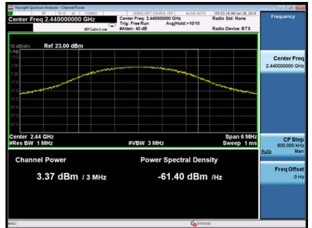
Zigbee, Carrier frequency (MHz): 2440
