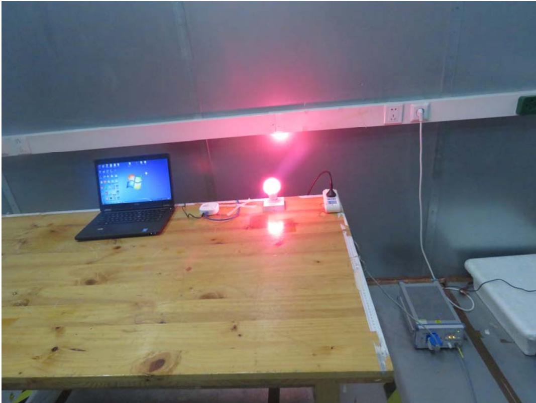
Picture 3 Conducted Emission Test Setup
