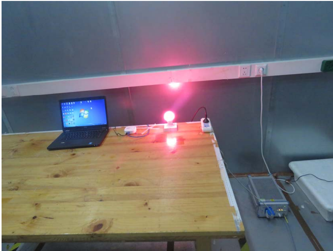
Picture 3 Conducted Emission Test Setup
