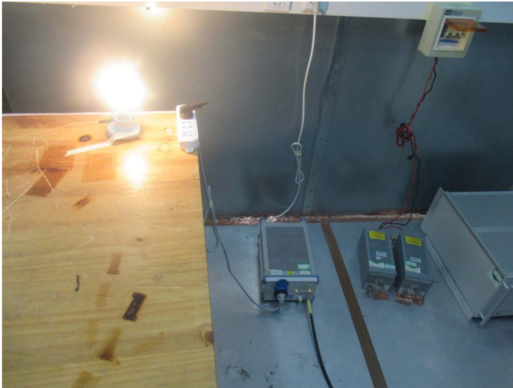
Picture 2 Conducted Emission Test Setup
