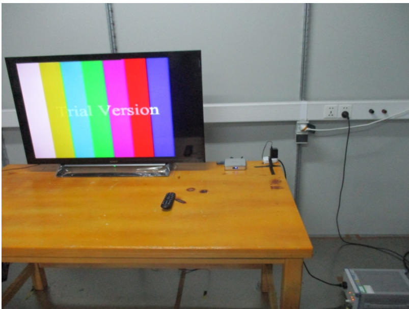
AC Power Line Conducted Emission
