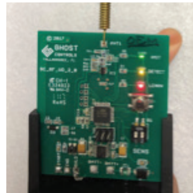
Example B. All LED's will turn ON for 1 second when the unit powers up and then will go OFF.
