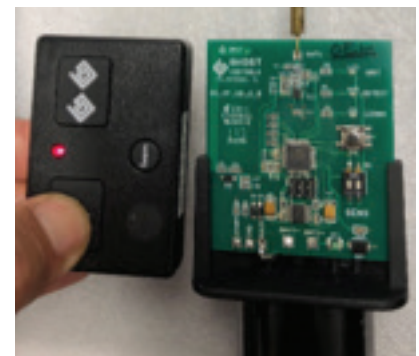
Example C. RED LED light on control board should go OFF. Now you can OPEN your gate with vehicle sensor
