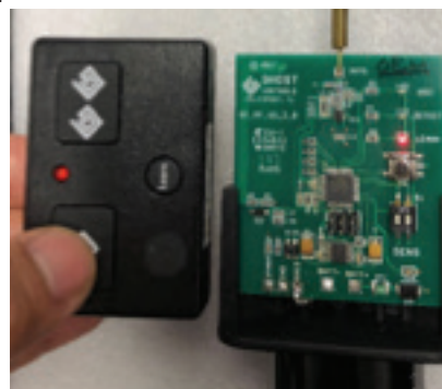
Example B. Place transmitter next to Control Unit Board. Press and hold the button that controls gate
