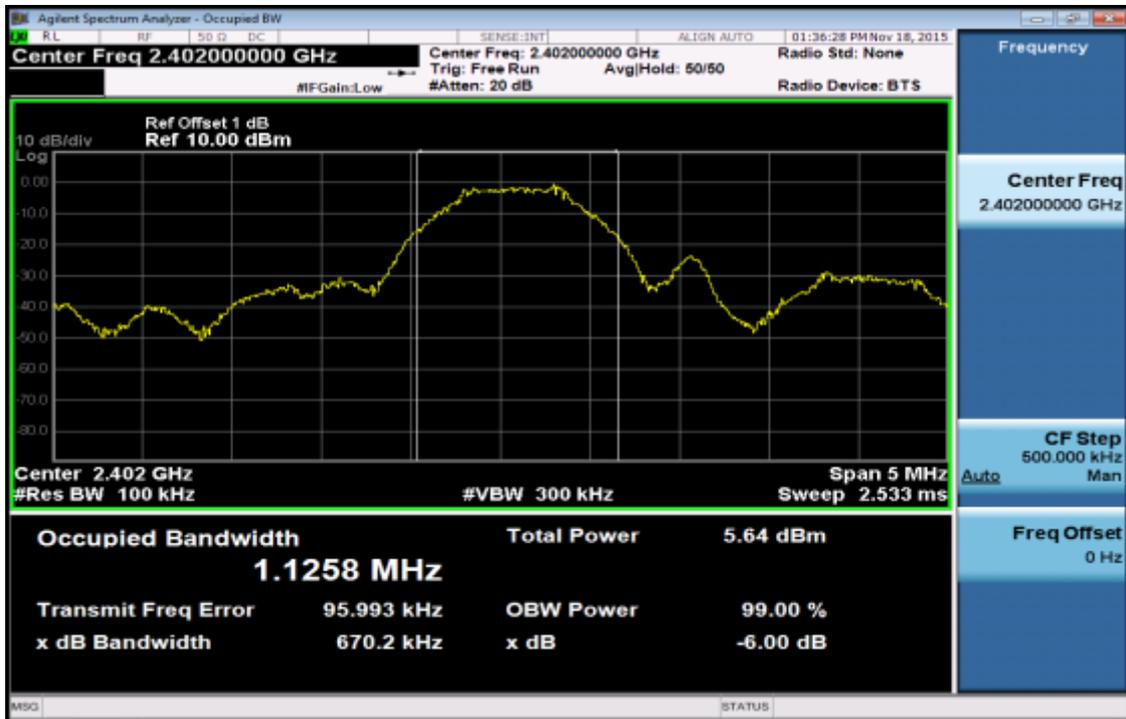
**6dB Band Width Test Data CH-Mid**
