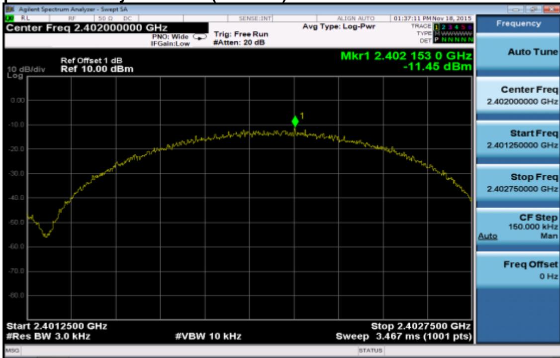
Power Spectral Density Test Plot (CH-Mid)
