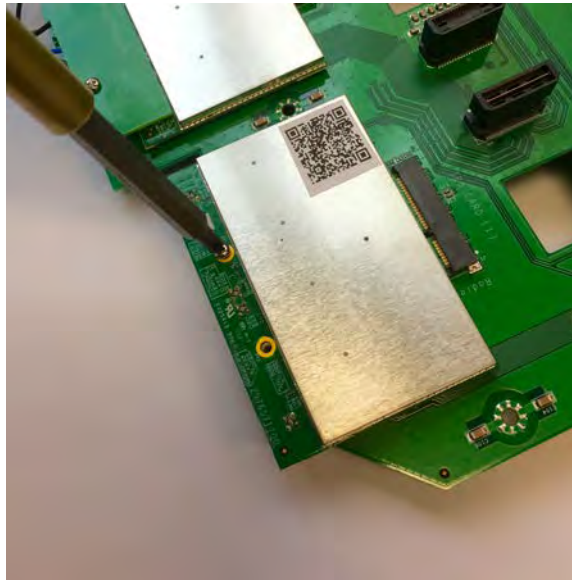
Figure 10 – Secure the 802.11ac WiFi Radio Module in to the PCIe card
