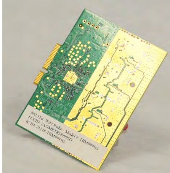
Figure 2 - Bottom View of the 802.11ac WiFi Radio Module - U.FL connectors
