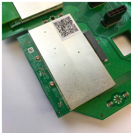
Figure 11 – Top View - Final Position of 802.11ac WiFi Radio Module on PCIe Card.
