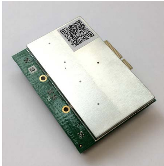
Figure 6 – Top View of the 802.11ac WiFi Radio Module - Samtec IP5 connectors
