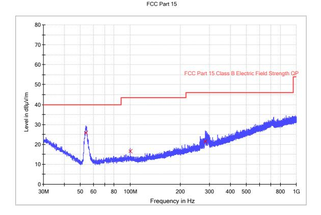
QuasiPeak Meas. Bandwidth Polarization Corr. Limit -Frequency Margin (MHz) (dBµV/m) Time (kHz) (dB) - QPK QPK (dB) (dBµV/m) (ms) 54.056000 25.7 1000.0 120.000 Н 8.1 14.3 40.0 100.001667 16.6 1000.0 120.000 Н 10.3 26.9 43.5 16.0 283.590333 21.4 120.000 Н 1000.0 24.6 46.0
