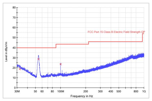
Frequency QuasiPeak Meas. Bandwidth Polarization Margin - QPK Limit -Corr. (dB) (dBµV/m) (kHz) QPK (MHz) Time (dB) (dBµV/m) (ms) 32.489667 18.6 1000.0 120.000 V 17.1 21.4 40.0 54.529067 28.7 1000.0 120.000 ٧ 8.1 11.3 40.0 100.001667 120.000 ٧ 23.6 1000.0 10.3 19.9 43.5
