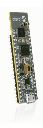
Flexible Form Factor Use Afero Modulo-2 standalone, or as a tool to enhance your MCU project. For hobbyists, Afero Modulo-2 attaches to a compatible Arduino® board (such as Uno) via the Afero Plinto shield, or to an Arduino Teensy development board directly.
