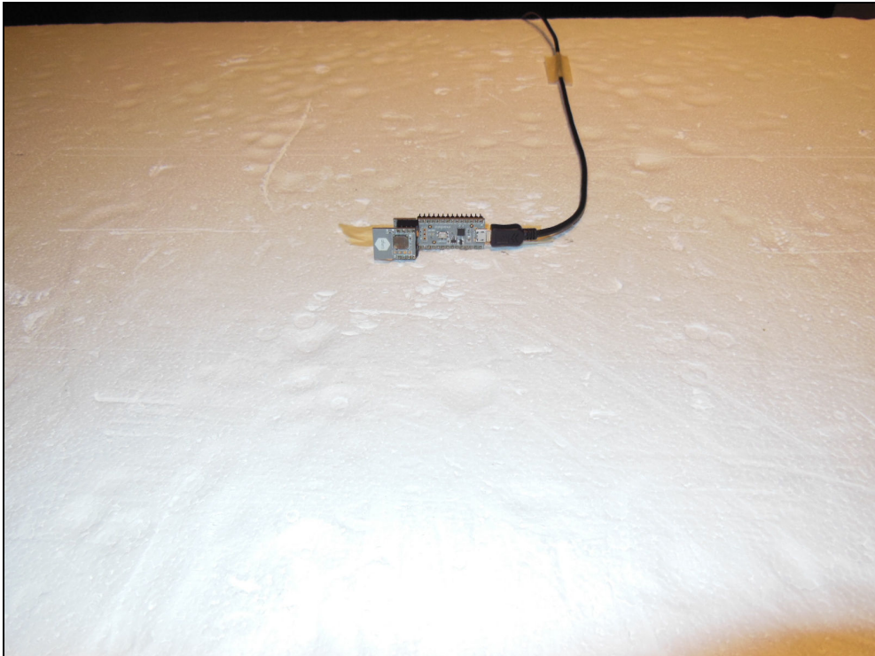
Figure 4: Radiated Emissions – Detached Eval Board
