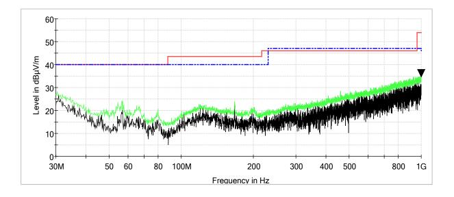
13.56 MHz: Characterization Scan, 30 MHz to 1000 MHz, Vertical
