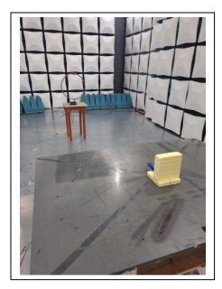
Radiated Spurious Emissions: Less than 30 MHz
