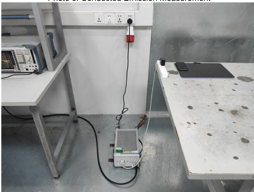
FCC ID: 2AGLG-TP007 Photo of Conducted Emission Measurement
