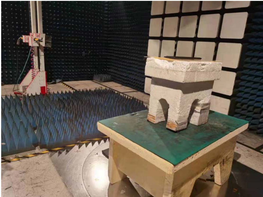
Spurious Emission Test Setup (Above 1GHz)
