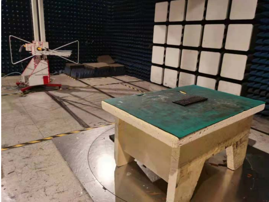
Spurious Emission Test Setup (Above 1GHz)
