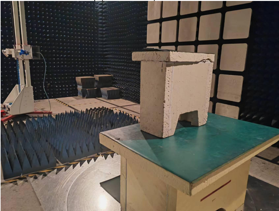
Spurious Emission Test Setup (30MHz-1GHz)
