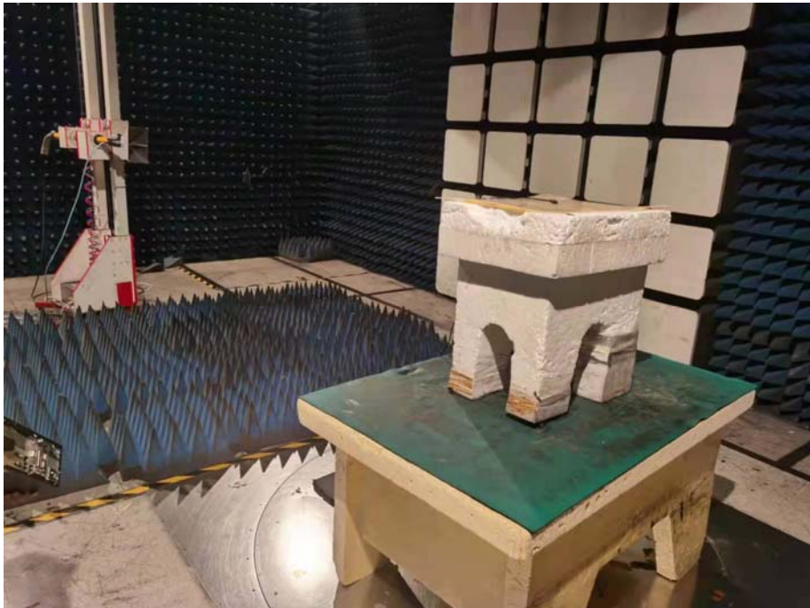
Spurious Emission Test Setup (Above 1GHz)
