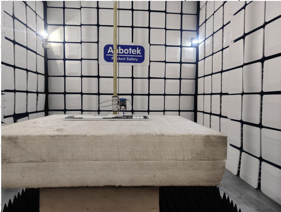
Photo of Radiation Emission Test (above 1GHz)
