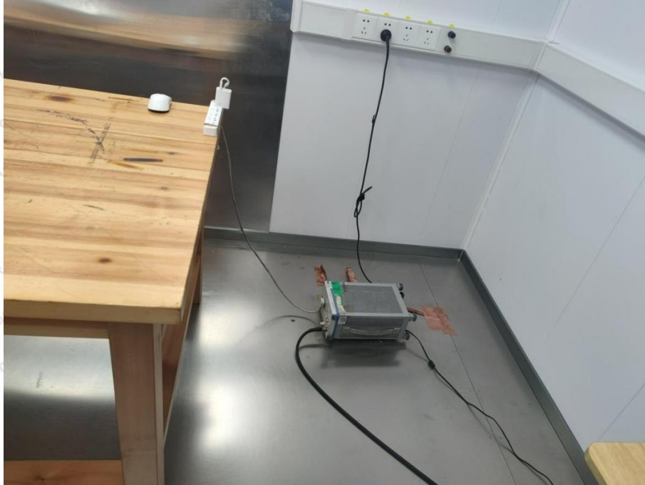
Conducted Emission at AC power line
