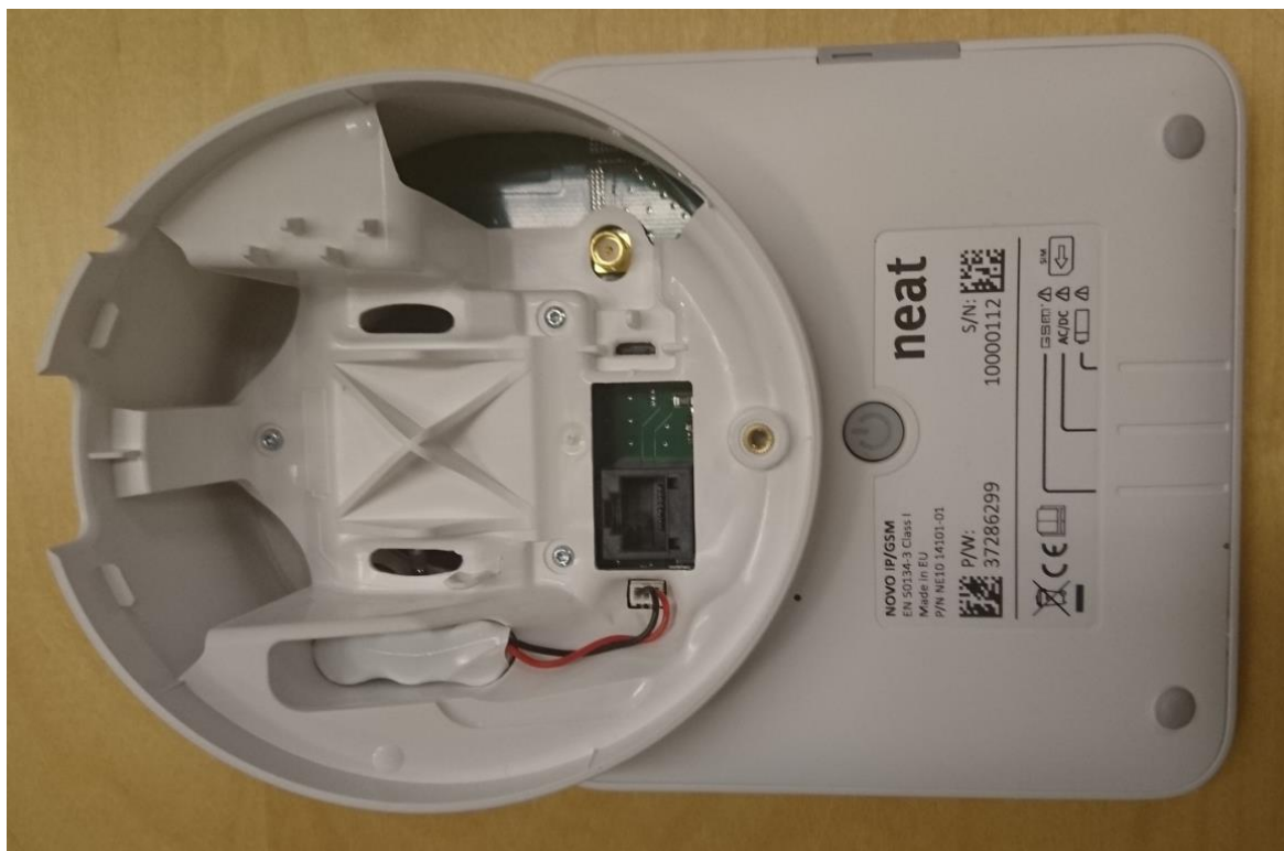
NOVO IP PLASTIC COVER, INSIDE LOUDSPEAKER AND BATTERY COMPARTMENT
