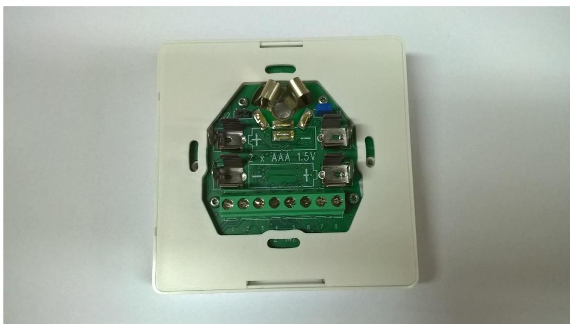
BACKSIDE VIEW OF DEVICE BASED ON PCB WITH 6.5 MM STEREO CONTACTED DEPOPULATED.
