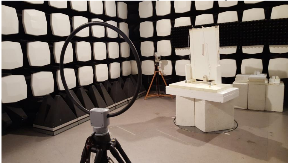
9 kHz-30 MHz, semi anechoic chamber, loop antenna, antenna pos A
