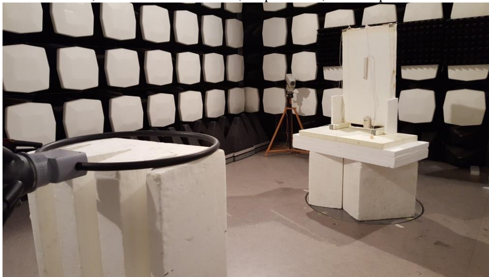
9 kHz-30 MHz, semi anechoic chamber, loop antenna, antenna pos C
