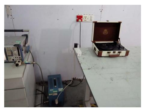
6.2 Radiated spurious emissions Test Setup(below 1GHz)
