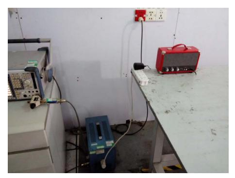
6.2 Radiated spurious emissions Test Setup(below 1GHz)
