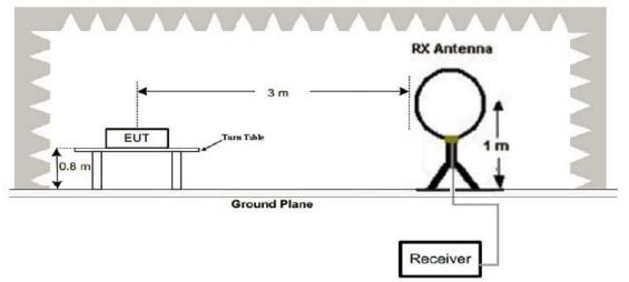
(2) Radiated Emission Test-Up Frequency 30MHz~1GHz
