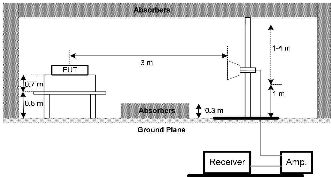
(C) For radiated emissions below 30MHz
