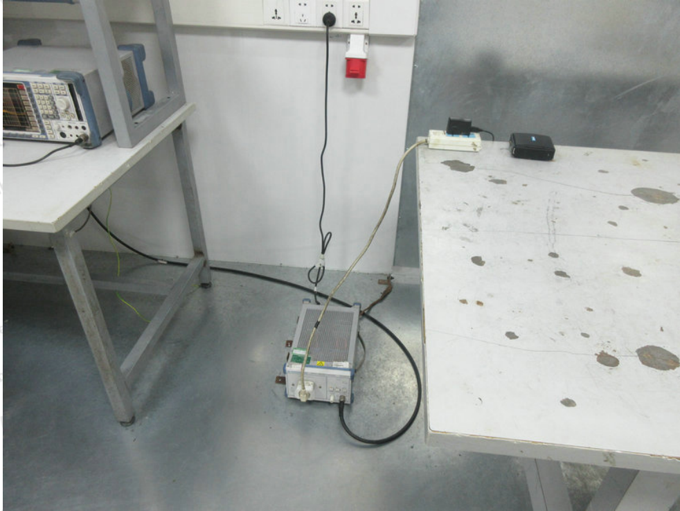
Photo of Power Line Conducted Emission Test
